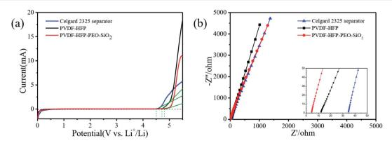
Fig. 4 (a) LSV curves and (b) impedance spectra of the Celgard 2325 separator absorbed liquid electrolyte and PVDF-HFP-based GPEs.
