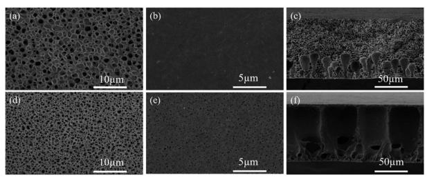
Fig. 1 SEM images of (a) bottom surface, (b) top surface and (c) cross section of PVDF-HFP membrane. SEM images of (d) bottom surface, (e) top surface and (f) cross section of PVDF-HFP-PEO-SiO<sub>2</sub> membrane.
