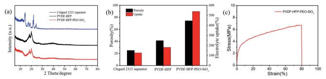
Fig. 3 (a) XRD patterns, (b) porosity and electrolyte uptake of the Celgard 2325 separator, pure PVDF-HFP and PVDF-HFP-PEO-SiO<sub>2</sub>, (c) stress-strain curve of the PVDF-HFP-PEO-SiO<sub>2</sub> GPE.
