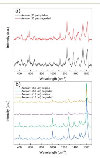
Fig. 3 Raman spectra of (a) pristine and degraded Aemion and (b) pristine and degraded Aemion+ membranes. Pristine samples were used as received from the manufacturer. Degraded samples were obtained after immersing previously counter-ion exchanged pristine samples in a solution consisting of  $0.1\,\mathrm{M\,VO_2}^+$ ,  $2\,\mathrm{M\,H_2SO_4}$  and  $100\,\mathrm{mM}$   $\mathrm{H_3PO_4}$  for over 1000 hours at 35 °C.
