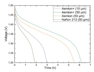
Fig. 4 Static self-discharge curves of Aemion (50 μm), Aemion+ (50  $\mu$ m), Aemion+ (15  $\mu$ m) and Nafion 212 (50  $\mu$ m) in a diluted (0.1 M) vanadium electrolyte.
