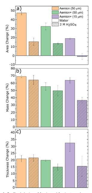
Fig. 1 Swelling behaviour of Aemion and Aemion+ membranes with sulfate counter-ions in water and 2 M  $\rm H_2SO_4$ . (a) Area change, (b) mass change and (c) thickness change are shown with clear bar charts representing samples immersed in water and shaded bar charts representing those immersed in 2 M  $\rm H_2SO_4$ . Wet values were taken from samples that were immersed in the appropriate liquid for 24 hours at room temperature (24 °C).
