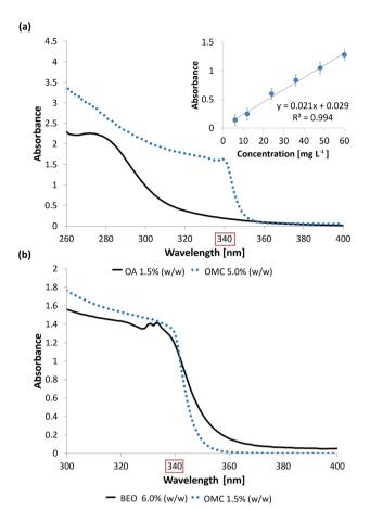
Fig. 2 (a) UV absorption spectra of a 1.5% (w/w) OA standard solution (black solid line) and a 5.0% (w/w) OMC standard solution (blue dotted line). The calibration curve for OMC at 340 nm and in the concentration range of 6.0-60.0 mg L<sup>-1</sup> is also shown. (b) UV absorption spectra of a 6.0% (w/w) BEO standard solution (black solid line) and a 1.5% (w/w) OMC standard solution (blue dotted line).
