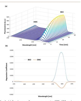
Fig. 4 (a) Synchronous fluorescence spectra (370–690 nm) corresponding to the central point of the experimental design registered as function of the permeation time (60 min). The emission band between 370 and 420 nm corresponds to OMC while the band between 570 and 650 nm corresponds to BEO. (b) First latent variable for PLS models corresponding to OMC (orange solid line) and BEO (blue dotted line).
