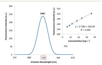
Fig. 3 Fluorescence spectrum corresponding to a standard solution of OMC (30 mg  $\rm L^{-1}$ ). The characteristic maximum of signal at 390 nm and the calibration curve in the concentration range of 6.0–36.0 mg  $\rm L^{-1}$  are shown. It is important to note that OA is not fluorescent around 390 nm.
