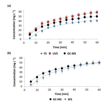
Fig. 5 Permeation profiles for OMC in the o/w microemulsions obtained using the proposed methodology and the reference method. (a) OMC permeation profiles corresponding to OMC-MEI obtained by UVS (red squares), FS (blue diamond) and GC-MS (black circle) methods. (b) OMC permeation profiles corresponding to OMC-MEII obtained by SFS (blue diamond) and GC-MS (black circle) methods. The experiments were performed in triplicate.
