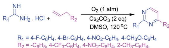
Scheme 5 Synthesis of polysubstituted pyrimidines via base-facilitated intermolecular oxidative C–N bond fabrication.
