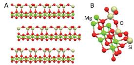
Fig. 9 X-ray structure of chrysotile,  $Mg_3(Si_2O_5)(OH)_4$ . (A) Layer structure, and (B) half of the unit cell (ICSD 41363). Mg, green; O, red; Si, cream.
