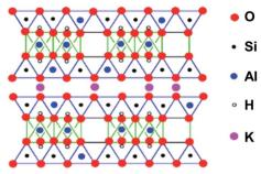
Fig. 7 The structure of a mica, muscovite,  $(KF)_2(Al_2O_3)_3(SiO_2)_6(H_2O)$ . The space between the layers is occupied only by  $K^+$  ions. The layer structure facilitates cleavage to produce flat surfaces. Adapted from https://employees.csbsju.edu/cschaller/PrinciplesChem/network/ NWalumina.htm (accessed  $17^{th}$  November 2020), courtesy of Chris Schaller
