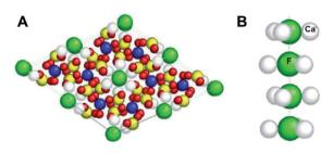
Fig. 5 X-ray crystal structure of fluorapatite, the phosphate mineral  $Ca_5(PO_4)_3F$ , showing (A)  $2\times 2$  unit cells, and (B) a column of  $F^-$  ions. Each  $F^-$  ion is bonded to  $F^-$  ions above and below it (F–F 3.44 Å) and to  $3 Ca^{2+}$  ions (F–Ca 2.463 Å) which form a triangle around it. Ca, grey; P, yellow; O, red; F, green. (A) is reproduced and (B) adapted from ref. 29 with permission from AO Research Institute Davos, copyright 2001.<sup>29</sup>
