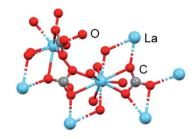
Fig. 10 X-ray crystal structure of  $La_2(CO_3)_3 \cdot 8H_2O$  (CCDC1599003).  $La^{3+}$  is 10-coordinate with coordination sites occupied by water, bidentate and monodentate carbonate, La-O bond lengths 2.52–2.74 Å. It is a layer structure with alternate rows of carbonate anions and lanthanide cations. A quarter of the water molecules are unbound and between layers. La, blue; O, red; C, grey. C0 (ICSD-22224).
