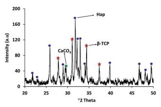
Fig. 3 XRD pattern of Hap synthesized by UV-excitation of eggshells.
