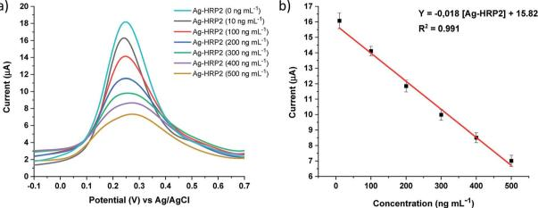
Fig. 6 a) DPV recorded with the Ab-PfHRP2/DHP/GE electrochemical immunosensor upon additions of Ag-PfHRP2 (10, 100, 200, 300, 400, and 500 ng mL<sup>-1</sup>), (b) calibration curve: Y = -0.018 [Ag-PfHRP2] + 15.82, with an  $R^2 = 0.991$ .
