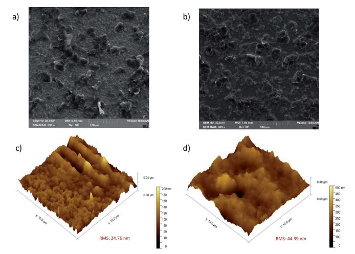
SEM and 3-dimensional AFM images: (a and c) DHP/GE surface, (b and d) Ab-PfHRP2/DHP/GE surface
