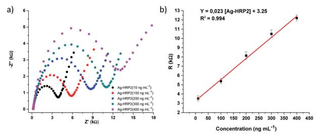
Fig. 5 (a) EIS spectra recorded with the Ab-PfHRP2/DHP/GE electrochemical immunosensor upon additions of Aq-PfHRP2 (10, 100, 200, 300, and 400 ng mL<sup>-1</sup>), (b) calibration curve: Y = 0.023 [Ag-PfHRP2] + 3.25, with an  $R^2 = 0.994$ .
