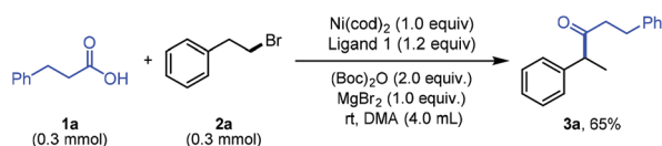
Scheme 2 Stoichiometric reaction without electric current.
