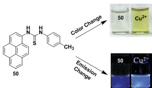
Fig. 44 The colour and fluorescence changes of chemosensor \mathbf{50} upon addition of \text{Cu}^{2+} ions. Reproduced from ref. 119 with permission from the Elsevier, copyright 2010.
