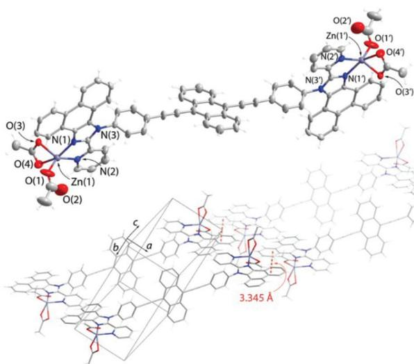
**Fig. 12** Molecular view and packing fragment of **3OAc<sub>y</sub>**. Crystallization solvent was disordered and omitted from the refinement model. The intermolecular  $\pi$ - $\pi$  distances were measured between the planes of the phenanthrene motifs. Symmetry transformations used to generate equivalent atoms ( $'$ ):  $-x, 1 - y, -z$ . Thermal ellipsoids are shown at the 50% probability level.
