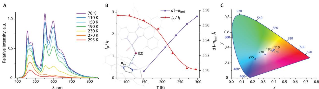
**Fig. 8** (A) Variable temperature solid state emission spectra of **1I\_b**; (B) temperature dependences of the ratio of intensities of the phosphorescence and fluorescence bands ( $I_p/I_f$ ), and of the intermolecular distance between the iodine atom and the plane of imidazole ( $d(I \cdots \pi_{imi})$ ); and (C) CIE 1931 coordinates of the emission of **1I\_b** at different temperatures.
