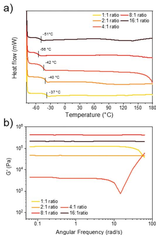
**Fig. 3** Thermal and rheological properties of  $C_6E-3T$  networks. (a) DSC thermograms of the 2nd heating cycle from  $-80$  to  $180$  °C,  $10$  °C  $min^{-1}$ . (b) Frequency sweep analysis of films showing storage modulus versus frequency at 25 °C (1% strain from 0.1 to 10 Hz, or 0.06 to 62  $rad\ s^{-1}$ ).
