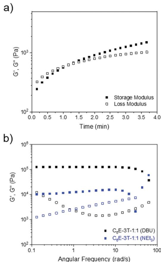
**Fig. 2** (a) Rheology time sweep (10% strain, frequency of 1 Hz) at 25 °C to characterise gelation time of  $C_6E-3T-1:1$  using 1 mol% DBU. (b) Frequency sweep analysis showing storage and loss modulus versus frequency for networks synthesized using DBU or  $NEt_3$  at 25 °C (1% strain from 0.1 to 10 Hz, or 0.06 to 62  $rad\ s^{-1}$ ).
