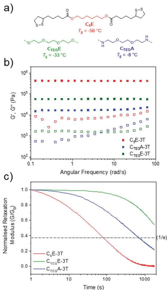
Fig. 4 (a) Structures of monomers to make networks at 8 : 1 ratio. (b) Rheology frequency sweep of networks at  $25$  °C (1% strain from  $0.1$  to  $10$  Hz, or  $0.06$  to  $62$   $\text{rad s}^{-1}$ ). (c) Stress relaxation experiments at 2% strain,  $100$  °C.
