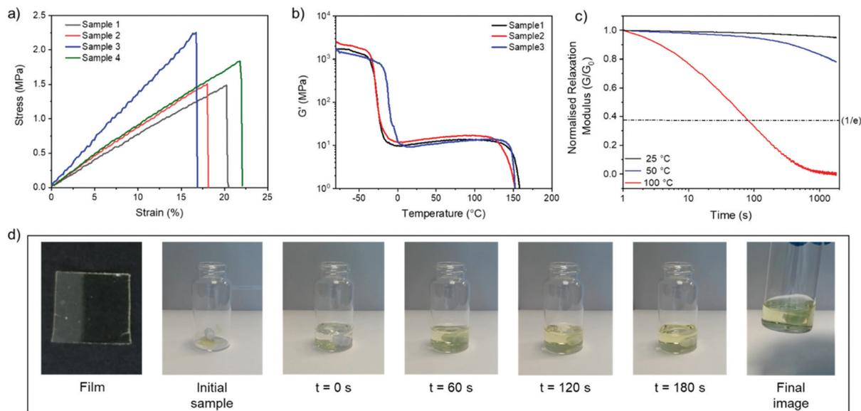
**Fig. 5** Thermomechanical and physical data for C6E-3T-8:1. (a) Uniaxial tensile testing at 22 °C, 10 mm min<sup>-1</sup> strain rate. (b) DMA temperature sweep from -80 to 180 °C, 5 °C min<sup>-1</sup>. (c) Stress relaxation experiments at 2% strain (25 °C, 50 °C, and 100 °C). (d) Chemical recycling of as-synthesised film cut into small pieces (200 mg film in 5 mL DCM solution, 0.01 M DBU).
