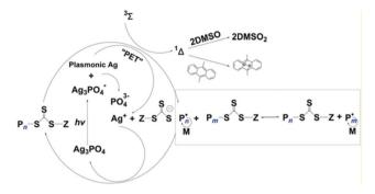
Fig. 8 Proposed mechanism of PET-RAFT catalyzed by  ${\rm Ag_3PO_4}$  and the singlet oxygen quenching pathway. Reproduced from ref. 95 with permission from Wiley-VCH Verlag GmbH & Co. KGaA, Weinheim, copyright 2019.
