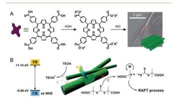
Fig. 15 Self-assembly of rod-like SA-TCPP and its use in PET-RAFT polymerization. Reproduced from ref. 153 with permission from Wilev-VCH Verlag GmbH & Co. KGaA, Weinheim, copyright 2020.
