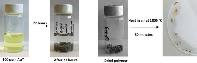
Fig. 4 Visual progress of  $Au^{3+}_{(aq)}$  extraction and  $Au^{0}$  recovery mediated by 100 mg of PtnPDL-CLP.  $[Au^{3+}]_{0} = 100$  ppm,  $Au^{3+}$  volume = 10 mL.
