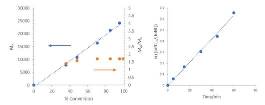
Fig. 2 (Left) M<sub>n</sub> versus conversion, and (Right) First-order evolution of [tnNL] versus time. Reaction conditions: tnNL (2 M, 0.632 mmol, 1 equiv.), benzyl alcohol (1 mol%, 0.0063 mmol) catalyzed by TCC/BEMP (5 mol%, 0.0315 mmol each) in  $C_6D_6$ .
