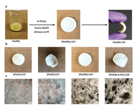
Fig. 3 (a) Image of PtnPDL-CLP flexible polymer. (b) Images of PtnCL, PtnHL, and P(tnPDL-b-CL) CLPs (c) Cross sectional morphology of cross-linked polymers under optical microscopy; magnification ×10.
