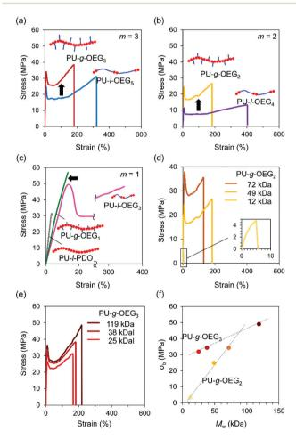
Fig. 3 Stress-strain curves for m = 3 system (PU-g-OEG<sub>3</sub> and PU-l- $OEG_5$ ) (a), m = 2 system (PU-g-OEG<sub>2</sub> and PU-l-OEG<sub>4</sub>) (b), m = 1 system  $(PU-g-OEG_1 \text{ and } PU-l-OEG_3)$  and PU-l-PDO (c) with various molecular weights for PU-g-OEG<sub>3</sub> (d), PU-g-OEG<sub>2</sub> (e), and plots for stress at break  $(\sigma_b)$  vs. the weight-average of molecular weight  $(M_w)$  (f) with a crosshead speed of 10 mm  $min^{-1}$  (n = 3).
