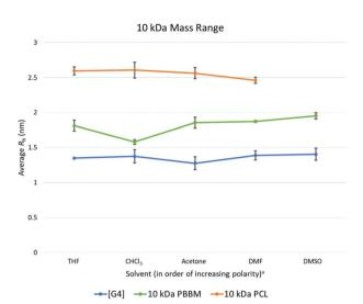
**Fig. 8** Calculated average  $R_{\rm h}$  values, from DOSY- $^{1}$ H NMR, for Tetra[G4] Bnz<sub>32</sub>, 10 kDa PCL, and 10 kDa PBBM in all tested solvents.  $^{\rm a}$  Solvent polarity values from Reichardt were used to determine order of polarity.  $^{39}$
