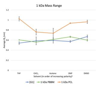
Fig. 5 Calculated average  $R_{\rm h}$  values, from DOSY- $^1$ H NMR, for Tetra[G1] Bnz<sub>4</sub>, 1 kDa PCL, and 1 kDa PBBM in all tested solvents.  $^a$  Solvent polarity values from Reichardt were used to determine order of polarity.  $^{39}$
