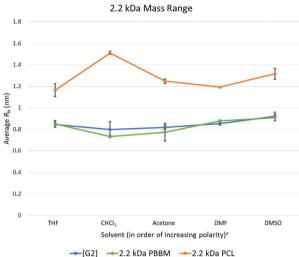
**Fig. 6** Calculated average  $R_{\rm h}$  values, from DOSY- $^{1}$ H NMR, for Tetra[G2] Bnz<sub>8</sub>, 2.2 kDa PCL, and 2.2 kDa PBBM in all tested solvents.  $^{\rm a}$  Solvent polarity values from Reichardt were used to determine order of polarity.  $^{39}$
