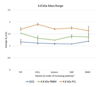
Fig. 7 Calculated average  $R_{\rm h}$  values, from DOSY- $^{1}$ H NMR, for Tetra[G3] Bnz<sub>16</sub>, 4.8 kDa PCL, and 4.8 kDa PBBM in all tested solvents.  $^{\rm a}$ Solvent polarity values from Reichardt were used to determine order of polarity.  $^{39}$
