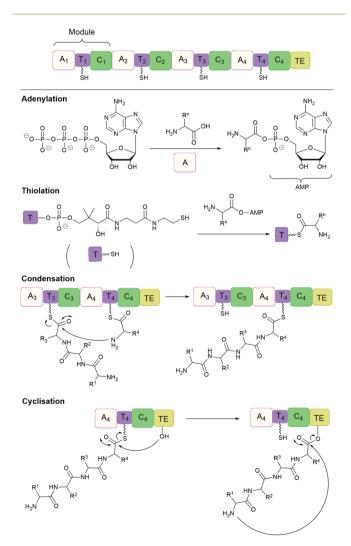
Fig. 7 Non-ribosomal peptide synthesis by NRPS modules composed of adenylation (A), thiolation (T) and condensation (C) domains with a terminal thioesterase (TE) domain.
