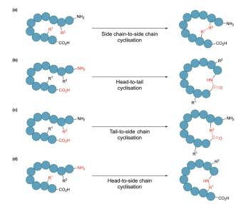
Fig. 1 Schematic illustration of cyclisation modes: (a) side chain-toside chain, (b) head-to-tail, also known as backbone cyclisation, (c) tailto-side chain, and (d) head-to-side chain.
