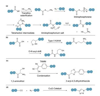
Fig. 4 Selected bioorthogonal reactions for peptide/protein cyclisation: (a) traceless Staudinger ligation, (b) type II KAHA ligation, (c) TAMM condensation, and (d) CuAAC.
