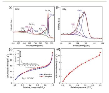
Fig. 5 (a) Co 2p and (b) S 2p XPS spectrum, (c) N<sub>2</sub> adsorption-desorption isotherms, and (d) CO<sub>2</sub> adsorption isotherm of Co<sub>9</sub>S<sub>8</sub> cages.
