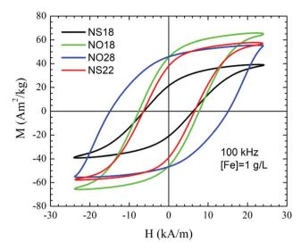
**Fig. 6** AC hysteresis loops obtained at 100 kHz and 24 kA m $^{-1}$  for water dispersions of samples NS18, NS22, NO18, and NO28 at a NP concentration of 1 g<sub>Fe</sub> l $^{-1}$ .
