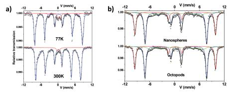
Fig. 3 (a) Representative 300 K and 77 K Mössbauer spectra of sample NS22 (blue: sextet, red: doublet, pink: quadrupolar component) and (b) Mössbauer spectra of samples NS22 and NO18 under an applied field of 8 T at 12 K.
