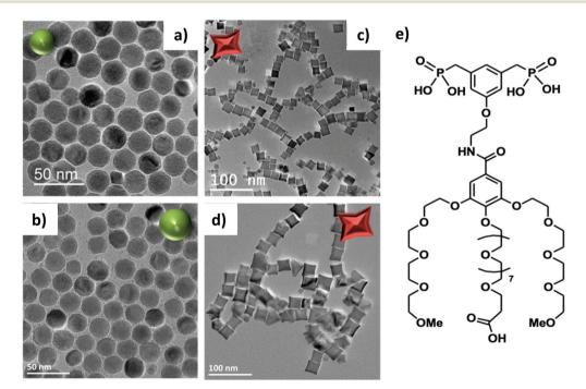
Fig. 1 TEM images of iron oxide NPs with different shapes and sizes: NS18 (mean size 17.2 ± 2 nm) (a), NS22 (mean size 22 ± 2 nm) (b), NO18 (17.2  $\pm$  2.2 nm) (c) and NO28 (27.8 $\pm$  4 nm) (d) and Scheme of the D2-2P dendron molecule (e).
