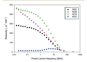
Fig. 7 NMRD profiles of the different NPs (NS10 corresponds to iron oxide NPs with a mean diameter of 10 nm and dendronized).
