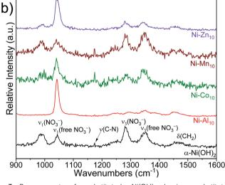
Fig. 3 Raman spectra of unsubstituted  $\alpha$ -Ni(OH)<sub>2</sub>, aluminum-substituted (Ni-Al<sub>10</sub>), cobalt-substituted (Ni-Co<sub>10</sub>), manganese-substituted (Ni-Mn<sub>10</sub>), and zinc-substituted ( $Ni-Zn_{10}$ ): (a) 350 cm $^{-1}$  to 600 cm $^{-1}$  spectral region and assignments of lattice modes; (b) 900 cm<sup>-1</sup> to 1600 cm<sup>-1</sup> spectral region and assignments of modes from compounds incorporated into the structure.
