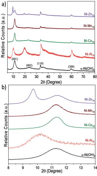
Fig. 2 X-ray diffraction of unsubstituted  $\alpha$ -Ni(OH)<sub>2</sub>, aluminum-substituted  $(Ni-Al_{10})$ , cobalt-substituted  $(Ni-Co_{10})$ , manganese-substituted  $(Ni-Mn_{10})$ , and zinc-substituted (Ni–Zn $_{10}$ ); (a) diffraction pattern with a  $2\theta$  scan range between 5-80°; (b) expanded region for a  $2\theta$  scan range between 8-14° showing changes of the (001) plane associated with the interlayer spacing of  $\alpha$ -Ni(OH)<sub>2</sub>
