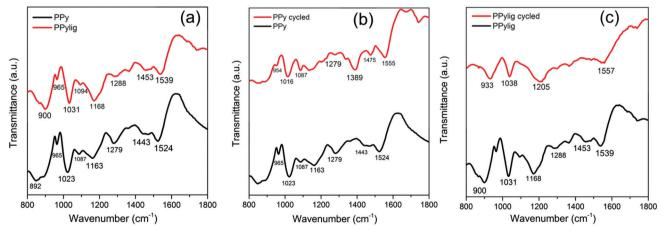
Fig. 6 (a) IR spectra of the electrodeposited polypyrrole (black line) and polypyrrole—lignin composite (red line), (b) comparison of polypyrrole (black line) and polypyrrole—lignin composite after cycling in a Zn-ion battery (red line).
