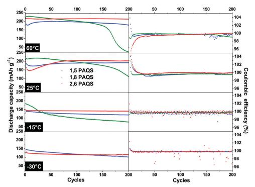
Fig. 7 Discharge capacities and corresponding coulombic efficiencies of **PAQS** isomers from 60  $^{\circ}$ C to -30  $^{\circ}$ C at 4C.
