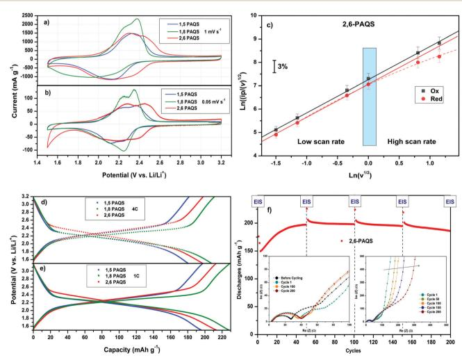
Fig. 4 (a) and (b) Cyclic voltammetry of PAQS isomers with 1 M LiTFSI in DOL/DME at 1.00 and 0.05 mV s<sup>-1</sup>. (c) Evolution of normalized current (ip) as a function of the square root of the scan rate v. (d) and (e) Galvanostatic profiles of each PAQS isomer at 4C and 1C. (f) 2,6-PAQS impedance evolution during galvanostatic cycling at 4C.
