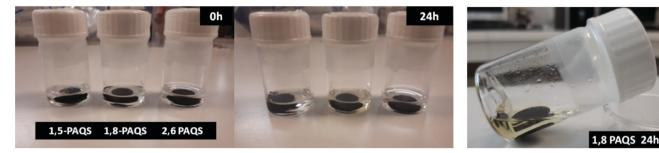
Fig. 3 Pictures showing the dissolution behavior of PAQS electrode materials in 1 M LiTFSI DOL/DME (1:1 v/v).
