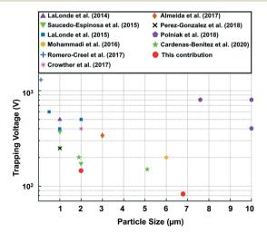
Fig. 6 Scatter plot comparing trapping voltage for different polystyrene particle size from previous works on insulator-based devices<sup>6,18–24</sup> and this contribution.
