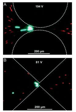
Fig. 7 Separation of a 6.8  $\mu$ m (green) and 2  $\mu$ m (red) particle mixture. (A) A separation of the mixture using a device with circular geometry, separation was achieved at 194 V. (B) Separation of the mixture using a device with triangular geometry, separation was achieved at 81 V.
