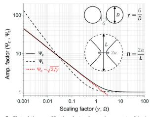
Fig. 3 Plot of the amplification factor for each geometry (bipolar or elliptic) as a function of the scaling factor ( $\gamma$  or  $\Omega$ , respectively). Scaling factors are schematically indicated in the inset figures. Geometric quantities are not drawn to scale.
