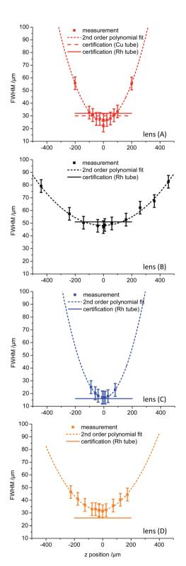
Fig. 3 FWHM values for Fe  $K_{\alpha}$  derived from knife edge scans on a razor blade in fluorescence mode for several positions along the X-ray beam focused by the polycapillary lenses. The measurement points were fitted by a second order polynomial to visualize the differences between the lenses. The horizontal lines depict the values derived from the certification, which are additionally listed in Table 3.
