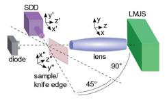
Fig. 1 Schematic μXRF setup. A polycapillary lens is placed in front of the LMJS. In  $90^{\circ}$  to the excitation path the energy dispersive SDD detector is placed and in 45° to the excitation and detection path the sample is placed. Polycapillary lens, detector and sample are placed on motorized stages for the alignment of the setup. A photo diode is placed in the excitation beam after the polycapillary lens for the alignment and to control the alignment during the measurements.
