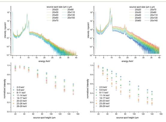
Fig. 5 Acceptance of the polycapillary lenses (left: lens (C), right: lens (A)). Top: Scattered excitation spectra measured in μXRF geometry using the plastic sample (i) and varied source spot sizes. Bottom: Integrated intensities concerning different energy regions (3 keV range) plotted against the varied source height. The region of 17 keV to 20 keV is excluded due to pile up effects of the Ga K lines.
