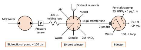
Fig. 1 Scheme of the fluidic manifold.
