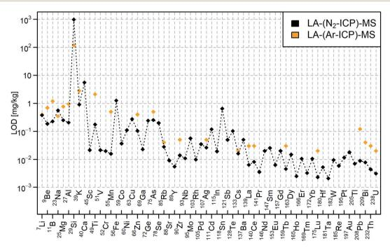
Fig. 4 LODs for NIST SRM 610 analyzed with LA-(N<sub>2</sub>-ICP)-MS (black) and LA-(Ar-ICP)-MS (orange) according to Günther et al.<sup>23</sup>
