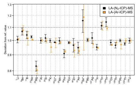
Fig. 5 Quantification of selected elements in NIST SRM 612 with LA-( $N_2$ -ICP)-MS (black) and LA-(Ar-ICP)-MS (orange) compared to their reference values<sup>38</sup> according to ESI, Table S4.† For the LA-(Ar-ICP)-MS measurement <sup>53</sup>Cr<sup>+</sup> and <sup>77</sup>Se<sup>+</sup> were used instead of <sup>52</sup>Cr<sup>+</sup> and <sup>78</sup>Se<sup>+</sup>. The confidence intervals were calculated based on four consecutive measurements with a confidence level of 95%.
