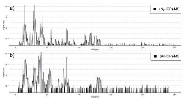
Fig. 2 Dry gas blank spectra of (a)  $(N_2-ICP)-MS$  and (b) (Ar-ICP)-MS. m/z 14 and 30 were not measured in the  $(N_2-ICP)-MS$  and m/z 40 and 41 were not measured in the (Ar-ICP)-MS to prevent detector saturation. The elevated noise in (b), especially in the range of m/z > 136, can be explained with the lower integration time leading to single detected ions causing a higher cps intensity.
