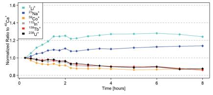
Fig. 6 Signal ratios to <sup>40</sup>Ca<sup>+</sup> normalized to the average of three NIST SRM 610 measurements after 15 minutes. Significant changes in signal ratios were observed in the first 1.5–2 hours. Afterwards, the signal ratios showed a stable trend with deviations below 5%.
