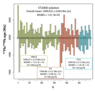
Fig. 4 Data compilation of apparent <sup>207</sup>Pb/<sup>206</sup>Pb dates from ET2000 synthetic solution at University of Geneva on TRITON TIMS, from Princeton University on PHOENIX TIMS, and from ETH Zürich TRITON Plus TIMS
