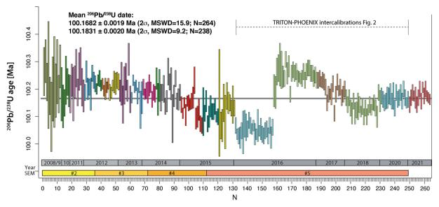
Fig. 1 Measurements of apparent <sup>206</sup>Pb/<sup>238</sup>U age from ET100 synthetic solution at UNIGE 2008–2015 on TRITON TIMS, 2016–2020 on both TRITON and PHOENIX TIMS, 2021 on PHOENIX only. TRITON data were measured using four subsequent secondary electron multipliers (#2 to #5). The color-coded blocks refer to blocks defined in Tables S1 and S2,† measurements #132-249 are shown in more detail in Fig. 2. See text for further details.
