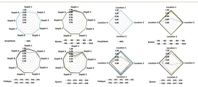
Fig. 2 Intra-mineral compositional variations of each mineral grain in sample M1, as assessed by comparing LIBS spectra taken at various locations and depths by the linear correlation function. The average spectrum across the non-varying coordinate, depth or location, was taken as reference during the comparisons. The ray plots show the correlation coefficient on their radial axes.
