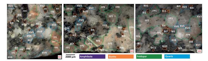
Fig. 1 Reflective optical microscopy images of the rock samples M1, M2 and M3 (Mórágy). The four studied mineral types are indicated in the images with abbreviations and borderline colours: AM = amphibole (purple), BI = biotite (orange), FP = feldspar (green), KV = quartz (blue). Individual laser sampling locations are indicated by red dots.
