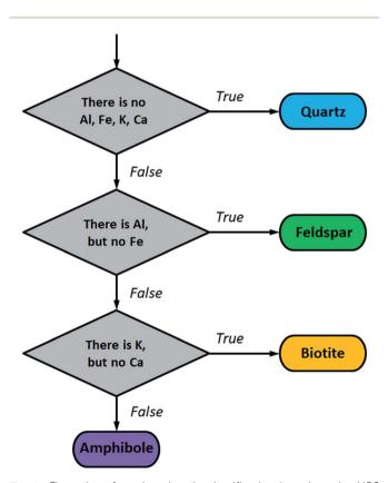
Fig. 4 Flow chart for mineral grain classification based on the LIBS detection of major components Al, Fe, K and Ca.
