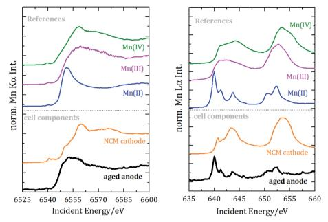
Fig. 4 Near-edge X-ray absorption spectrometry of manganese for the K-edge (left) and the L<sub>2</sub> und L<sub>3</sub> edges (right). Spectra are vertically shifted for better visualization
