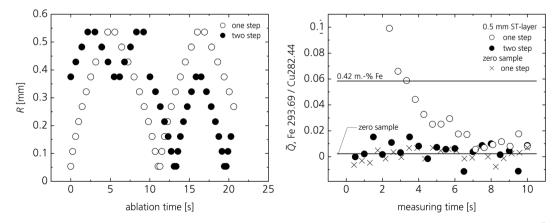
Fig. 7 Radial displacement R (left) of the laser beam as a function of time during the ablation phase and the resulting line ratio  $\tilde{Q}_{\text{Fe}}$  values during the measurement phase (right). Open symbols denote the one step ablation scheme, filled symbols denote the two-step scheme, see Fig. 6. For each data point shown in the right diagram an ablation sequence of 20 s was preceding as shown on the left.
