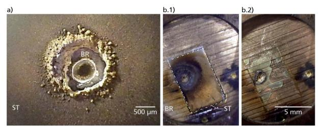
Fig. 2 (a) Crater caused by the DPO measurement inside of a previously pierced steel sheet (ST, see Fig. 1(a)). The brass block (BR), i.e. the substrate, was shifted prior to the measurement to place an unaffected area underneath the generated hole in the ST. (b.1) ST mounted on the BR. The contour of the ST is marked by a dash-dotted line; (b.2) as (b.1) after removal of the ST. The thickness of the ST is 0.5 mm.
