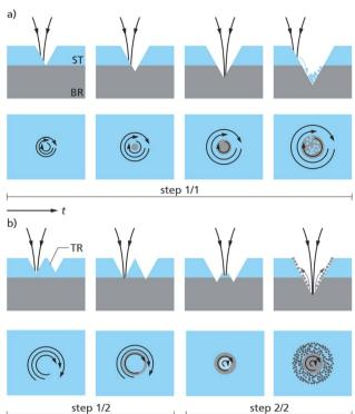
Fig. 6 Sketches of the cross-section and top view of the measuring object (see Fig. 1) for different ablation schemes: (a) one-step ablation and (b) two-step ablation. TR trench. Circular arrows indicate schematically the scan trajectories of the laser beam in the top views. Material of the ST is shown in light blue, and the material of the BR in grey.
