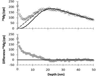
**Fig. 8** Illustration of DLC surface correction using measured data (circles, SW\_3) vs. SRIM best fit (solid line) for the first 50 nm of the <sup>24</sup>Mg depth profile. Top: comparison of raw data with the SRIM best-fit curve; dashed line gives an example of a (previously used<sup>10</sup>) visual correction based only on curve shape. Bottom: the difference between SRIM and the raw SIMS data.
