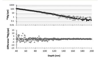
Fig. 7 Graphs demonstrating the quality of SRIM-fit to a measured DLC profile (SW\_3) for the last 160 nm of the <sup>24</sup>Mg depth profile. Top: raw data (circles) plotted with SRIM best–fit curve (line); bottom: the difference between SRIM and the raw SIMS data.
