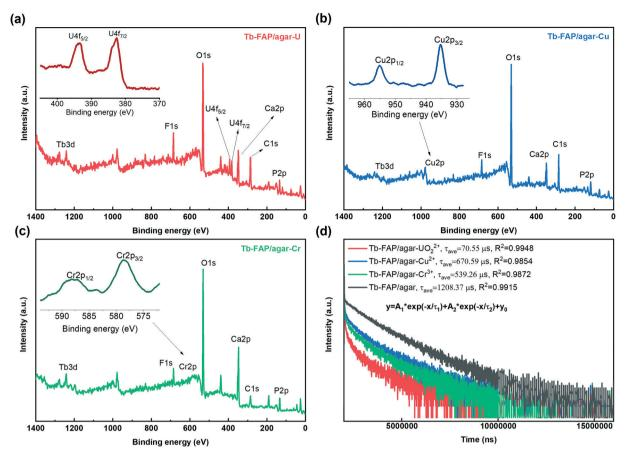
Fig. 4 XPS spectra of the Tb-FAP/agar after treatment with (a)  $UO_2^{2+}$ , (b)  $Cu^{2+}$ , and (c)  $Cr^{3+}$  accompanied with the insets showing the detailed XPS spectra of U 4f, Cu 2p, and Cr 2p, respectively. (d) The luminescence lifetime spectra of the Tb-FAP/agar sample recorded in the presence and absence of Cu<sup>2+</sup>, Cr<sup>3+</sup>, and UO<sub>2</sub><sup>2+</sup> ions ( $\lambda_{ex}$  = 377 nm and  $\lambda_{em}$  = 543 nm).
