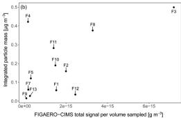
Fig. 4 Relationship between (a) total signal from organic compounds of each FIGAERO-CIMS sample and organic mass sampled by AMS aggregated to the filter sampling periods, (b) total signal of each FIGAERO-CIMS aerosol sample and the integrated particle mass of submicron aerosol aggregated to the filter sampling periods. F1–F13 are the sample numbers.
