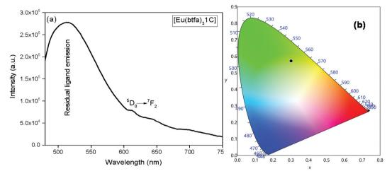
Fig. 5 (a) Emission spectrum in DCM at RT at 464 nm, (b) CIE-1931 chromaticity diagram demonstrating the calculated color coordinate (x, y) values for [Eu(btfa)31c] complex.
