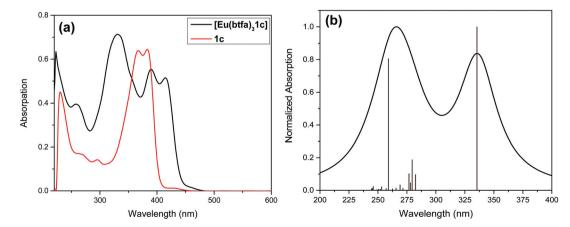
Fig. 2 (a) Optical absorption spectra of 1c and [Eu(btfa)31c] at RT. (b) Theoretical electronic spectrum calculated at the CAM-B3LYP level of theory using the B3LYP geometry for [Eu(btfa)31c].
