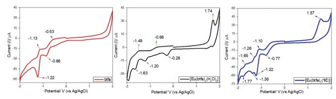
Fig. 7 Cyclic voltammograms of btfa (red), [Eu(btfa)<sub>3</sub>(H<sub>2</sub>O)<sub>2</sub>] (black) and [Eu(btfa)<sub>3</sub>1c] (blue) in the region between -2.0 to 2.0 V on glassy carbon electrode in 0.1 M Bu<sub>4</sub>NPF<sub>6</sub> solution in DCM at a scan rate of 100 mV s<sup>-1</sup>.
