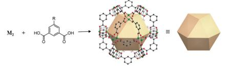
Fig. 23 Schematic illustration of the general design of  $\mathbf{cuo}$ -MOPs with  $M_2$  SBUs and 5-R-mBDC. M, green; C, black; O, red; all hydrogen atoms and solvents ligated on the metals are omitted for clarity.
