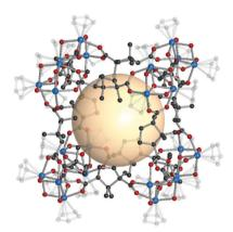
Fig. 17 Structural illustration of HCCF-1, [Cp<sub>3</sub>Zr<sub>3</sub>O(OH)<sub>3</sub>]<sub>8</sub>(**B59**)<sub>12</sub>.<sup>47</sup>
