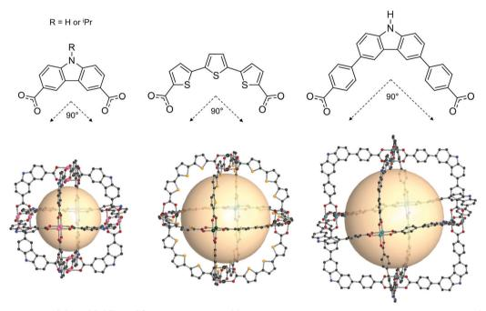
Fig. 14 Chemical diagram of B4 and B5, B7, and B8 ligands, which have 90° bent angles, and an architectural illustration of the oct MOPs resulting from the combination of M2 nodes and each linker. 72,73,78
