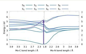
Fig. 10 Potential energy curves along a Mo-CO (left) and a Mo-NO (right) bond elongation yielding a bond dissociation energy of 1.12 eV for CO and 3.38 eV for NO dissociation (CASSCF(8,10)/ANO-RCC-MB; gas phase). Arrows indicate a possible photo-induced dissociation pathway
