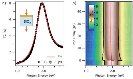
Fig. 1 (a) Steady state TC contrast spectra of monolayer WS<sub>2</sub> on thick FS substrate (black trace). Best fit using eqn (3) (red trace). (b) False color plot of the tr-TC as a function of probe photon energy (horizontal) and the pump-probe delay (vertical axis). The extracted fit parameter of exciton energy (red trace) and linewidth broadening (distance between black traces) obtained from fitting the time-dependent TC with egn (4) are overlaid on the same axis.
