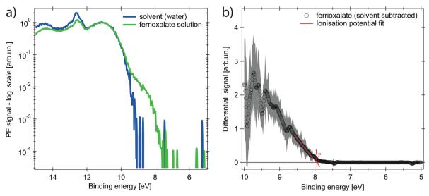
Fig. 2 Steady-state photoelectron (PE) spectra ( $h\nu = 37.2$  eV). (a) Solution of agueous ferrioxalate (green, 0.5 molar) and pure water solvent (blue), plotted on a logarithmic scale and normalised to the 1b<sub>1</sub> band of water at 11.16 eV. (b) Differential spectrum showing the ferrioxalate HOMO band only, whose ionisation potential is  $I_P = (7.9 \pm 0.2)$  eV. Experimental uncertainty of  $2\sigma$  as shaded grey area around the trace
