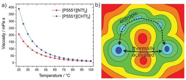
Fig. 12 (a) The ionic liquid with the more rigid anion, [P5551][CHTf<sub>2</sub>], has an almost twofold viscosity at room temperature compared to the ionic liquid with flexible anion, [P5551][NTf<sub>2</sub>]. <sup>140</sup> (b) The viscosity difference decreases with increasing temperature, which can be explained with basin theory, as more and more pathways become thermally activated. 180,378
