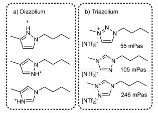
Fig. 22 Targeted modifications of the  $[C_4C_1im]^+$  cation: (a) diazolium based cations and (b) triazolium cations. Some properties for ionic liquids with triazolium [NTf2] ionic liquids have been measured, viscosities at 25 °C are given in (b). Values are taken from: 2-triaz viscosity, 285 4-triaz viscosity,<sup>283</sup> 5-triaz viscosity;<sup>284</sup> for the sake of simplicity we follow the numbering of the 1-butyl-3-methylimidazolium base structure.
