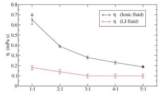
Fig. 6 Size differences can fluidize ionic liquids. The effect is less pronounced for the (uncharged) Lennard-Jones fluid. Reprinted from ref. 110, with the permission of AIP Publishing.
