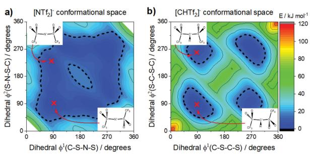
Fig. 11 The [NTf<sub>2</sub>]<sup>-</sup> anion (a) is extremely flexible, easily changing between *cis* and *trans* conformers. In contrast, replacing the imide nitrogen with a methanide group leads to the rigid  $[CHTf_2]^-$  anion (b), which experiences a high barrier for cis-trans interconversion. (a) and (b) adapted from ref. 140 -Published by the PCCP Owner Societies.
