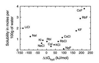
**Fig. 4** The solubility of simple alkali halides in water can be rationalised with size differences. Reprinted from J. Gujt, M. Bešter-Rogač and B. Hribar-Lee, *J. Mol. Liq.*, **190**, 34–41, Copyright 2014, with permission from Elsevier.
