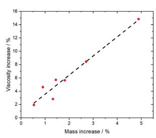
Fig. 5 The comparison of isotopologues with different mass reveals a correlation between viscosity and mass for a variety of different ionic liquids. Experimental data points from ref. 102, the dashed line is a linear fit.
