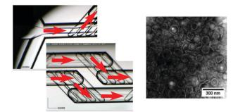
Fig. 8 Optical microscopy images of the microfluidic chip, with a simple cross-flow junction and mixing chambers (left, red arrows indicating the direction of flow), used in the self-assembly of pH responsive polymersomes (right, TEM image), adapted with permission from Albuquerque et al., Langmuir, 2019, **35**, 25, 8363–8372. Copyright (2019) American Chemical Society. 103
