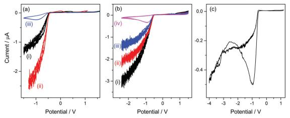
Fig. 2 CVs of a Pt ME in [bsmim]HSO<sub>4</sub> at 80 °C. (a) CVs in [bsmim]HSO<sub>4</sub> purified with two extraction steps (i), in crude [bsmim]HSO<sub>4</sub> (ii), and in [bsmim]HSO<sub>4</sub> purified with six extraction steps (iii). (b) CVs in crude [bsmim]HSO<sub>4</sub> (i), and after three successive additions (18 mg each) of pure Zbsmim (ii–iv). (c) Highly cathodic CV in [bsmim]HSO<sub>4</sub> purified with six extraction steps. T = 80 °C; v = 0.1 V s<sup>-1</sup>.
