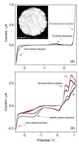
Fig. 1 CVs of a Pt microelectrode in [bmim]Br (a) and in [bmim]HSO<sub>4</sub> (b) before (i) and after (ii) addition of pure [bmim]Br. Inset in (a) shows a SEM picture of the Pt microelectrode after the voltammetric analysis (scale bar: 8  $\mu$ m).  $T = 80 \, ^{\circ}$ C;  $v = 0.1 \, \text{V s}^{-1}$ .
