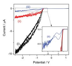
Fig. 3 CVs of a Pt ME in [bsHim]HSO<sub>4</sub> before (i) and after one (ii) and two (iii) additions of 15 mg of pure ZbsHim. Inset graph shows an expanded current scale over the potential interval  $-2.5 \text{ V} \leq E \leq 0.0 \text{ V}$ .  $T = 80 \,^{\circ}\text{C}$ ;  $v = 0.1 \text{ V s}^{-1}$
