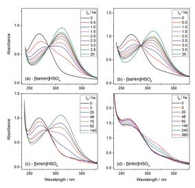
Fig. 4 UV-vis spectra of the reaction media for the transesterification reaction of **PNPA** with MeOH at 25 °C in the presence of **[bsmim]HSO<sub>4</sub>** (a), **[bsHim]HSO<sub>4</sub>** (b), **[bmim]HSO<sub>4</sub>** (c), and **[bHim]HSO<sub>4</sub>** (d), acquired at different  $t_R$  values, as indicated in each graph.
