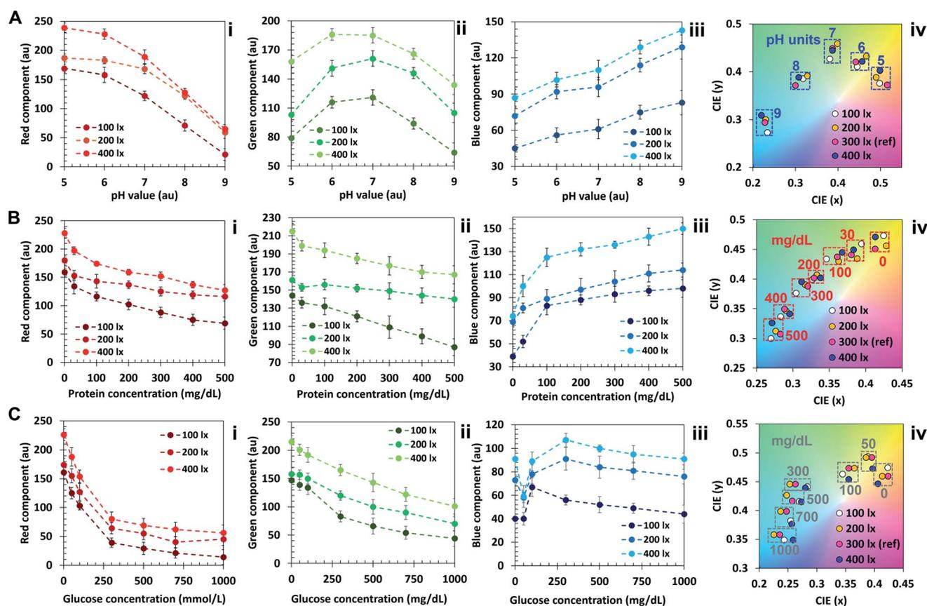
Fig. 5 Influence of ambient lighting on color recognition (100–400 lx). (A) Characterization of the pH sensor under 100–400 lx. (i) Red component; (ii) green component; (iii) blue component; (iv) CIE plot. (B) Characterization of the protein sensor under 100–400 lx. (i) Red component; (ii) green component; (iii) blue component; (iv) CIE plot; (C) characterization of the glucose sensor under 100–400 lx. (i) Red component; (ii) green component; (iii) blue component; (iv) CIE plot.
