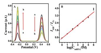
Fig. 4 (A) ACV profiles of this platform for the detection of miRNA with the concentrations of 0, 1 fM, 10 fM, 100 fM, 1 pM, 10 pM, 100 pM, and 1 nM (from a to h). (B) Calibration curve of  $I_{MB}/I_{Fc}$  vs. the logarithm of target miRNA concentration. Error bars represent standard deviations of three parallel tests.
