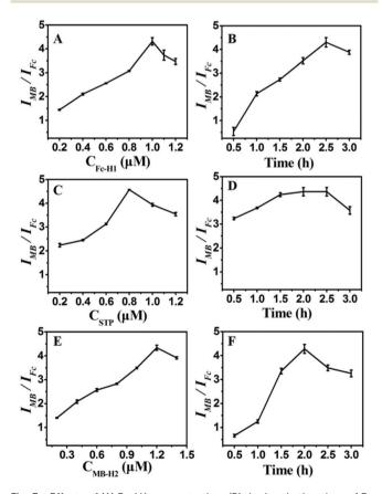
Fig. 3 Effects of (A) Fc-H1 concentration, (B) the incubation time of Fc-H1, (C) probe STP concentration, (D) the incubation time of probe STP, (E) MB-H2 concentration and (F) the incubation time of MB-H2. Error bars represent standard deviations of three parallel experiments.
