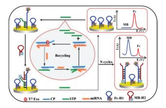
**Scheme 1** Schematic of the dual-signal ratiometric electrochemical biosensor based on the T7 Exo-assisted target recycling coupling nonenzymatic catalytic hairpin assembly for the detection of miRNA-141.
