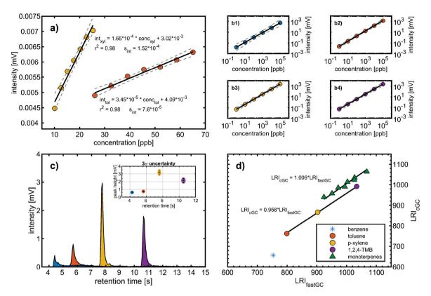
Fig. 2 Analytical figures of merit comprising (a) calibration functions of toluene (T) and p-xylene (X) with a coefficient of determination  $r^2$  and residual standard deviation  $s_{int}$ , (b1-b4) linearity over five orders of magnitude, (c) peak shape and precision (3 $\sigma$ ) of intensity and retention time from repeated BTXT analysis, and (d) comparison of the LRI obtained from fastGC with the LRI obtained from cGC for BTXT and 8 monoterpenes.
