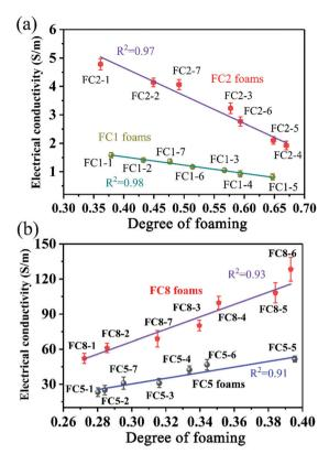
Fig. 4 The relationship of EC and degree of foaming for (a) FC1 foams and FC2 foams, and for (b) FC5 foams and FC8 foams.
