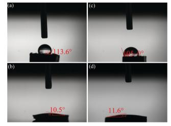
Fig. 10 (a) Water droplet and (b) methyl-silicone oil droplet placed on the outside of the FC5-5 composites. (c) Water droplet and (d) methyl-silicone oil dropped on the outside of the FC8-6 composites.
