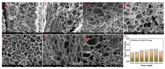
Fig. 3 SEM images of the cryo-fractured FC8 nanocomposite foams: (a) FC8-1, (b) FC8-2, (c) FC8-3, (d) FC8-4, (e) FC8-5, (f) FC8-6 and (g) FC8-7 samples. (h) Various FC8 foams' degree of foaming.
