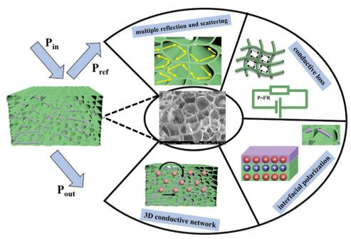
Schematic illustration of EM wave transmission across the PVDF/MWCNT nanocomposite foams and its related shielding mechanism.
