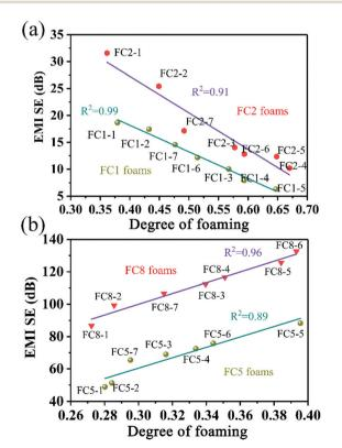
Fig. 7 The correlation between the mean SE<sub>T</sub> values and the degree of foaming for: (a) FC1 and FC2 foams, and (b) FC5 and FC8 foams.
