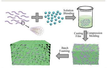
$\begin{tabular}{ll} Fig. 1 Schematic diagram for the fabrication process of the PVDF/MWCNT nanocomposite foams. \end{tabular}$
