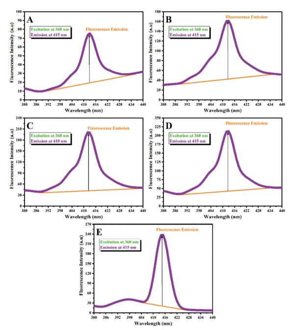
Fig. 6 Fluorescence emission spectra of the stimuli-chromic latex nanoparticles (with a solid content of about 0.3 wt%) excited at the wavelength of 360 nm: (A) PBA-SP, (B) PBAMMA-SP1, (C) PBAMMA-SP2, (D) PBAMMA-SP3, and (E) PMMA-SP.
