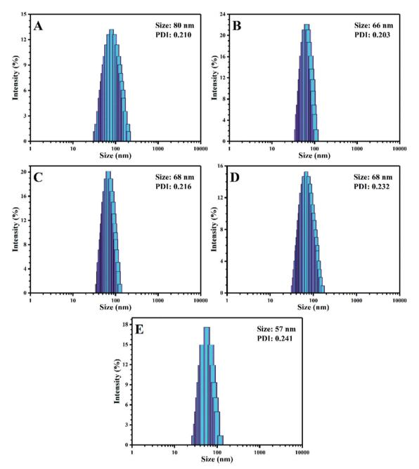
DLS results for the stimuli-chromic latex nanoparticles: (A) PBA-SP, (B) PBAMMA-SP1, (C) PBAMMA-SP2, (D) PBAMMA-SP3, and (E) PMMA-SP.
