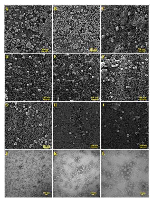
Fig. 4 SEM images for the stimuli-chromic latex nanoparticles: (A and B) PBA-SP, (C) PBAMMA-SP1, (D and E) PBAMMA-SP2, (F and G) PBAMMA-SP3, and (H and I) PMMA-SP. (J-L) TEM images of the stimuli-chromic latex nanoparticles (PMMA-SP) at different magnifications.
