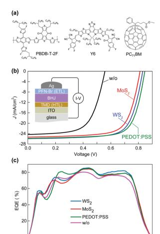
Fig. 3 (a) Molecular structures of PBDB-T-2F, Y6 and PC<sub>71</sub>BM. (b) J-Vcurves of PBDB-T-2F:Y6:PC71BM based OSCs without a HTL (w/o) and with WS2, MoS2 and PEDOT:PSS as the HTL. Inset: Schematic of the cell architecture. (c) EQE spectra of the cells shown in (b).
