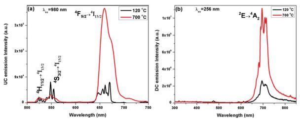
Fig. 4 (a) UC and (b) DC emission spectra of the ZGO-YEC-AP and ZGO-YEC-700 NPs under 980 nm and 254 nm excitation, respectively
