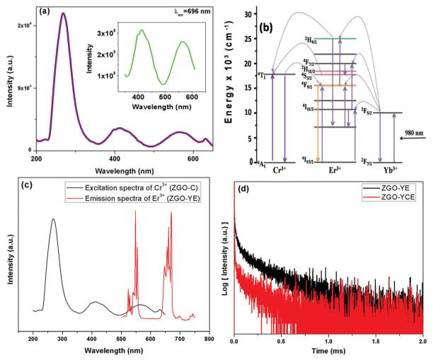
Fig. 5 (a) Excitation spectrum of the ZGO:Cr NPs, (b) proposed mechanism of the ET between dopants of the ZGO-YEC NPs, (c) spectral overlap between the Er<sup>3+</sup> emission of the ZGO-YE NPs and the Cr<sup>3+</sup> excitation of the ZGO-C NPs, and (d) decay profiles of Er<sup>3+</sup> ( $^4$ S<sub>3/2</sub>:  $\lambda_{em}$  = 560 nm) of the ZGO-YE and ZGO-YEC NPs.
