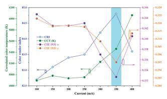
Fig. 9 The colorimetric parameters of Pr02Mn08 under blue LED excitation as a function of the driving current.
