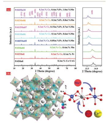
Fig. 1 XRD patterns of (a) TCs with different Pr3+ and Mn2+ doping concentrations and magnified XRD patterns around 33°, (b) schematic of the crystal structure of the Ce,(Pr,Mn):YAG TCs.
