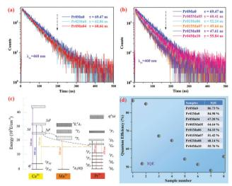
Fig. 8 Fluorescence decay curves: (a) Pr0Mn0, Pr02Mn0, Pr0Mn04. (b) PrOMnO, PrO05MnO5, Pr01MnO6, Pr015MnO7, Pr02MnO8, Pr04Mn10. (c) Schematic of the energy transfer process among Ce<sup>3+</sup>-Pr<sup>3+</sup>-Mn<sup>2+</sup> ions. (d) Internal quantum efficiencies (IQEs) of the TCs under 460 nm excitation
