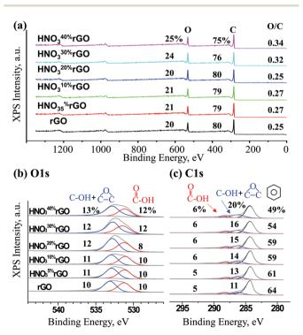
Fig. 5 XPS spectra of the initial and HNO<sub>3</sub>-treated rGO materials.
