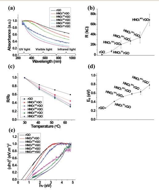
Fig. 3 (a) UV-vis spectra, (b) average resistance at 64 °C, (c) normalized resistance as a function of temperature from 30 to 64 °C, and (d) band gap energy for the initial and HNO3-treated rGO materials, and (e) Tauc plot for optical band gap determination.
