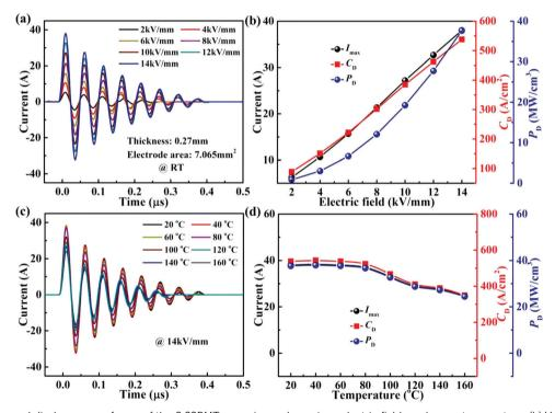
Fig. 9 (a) Underdamped discharge waveforms of the 0.22BMT ceramics under various electric fields and room temperature. (b) Variations of  $I_{\text{max}}$ ,  $C_{\text{D}}$ , and PD as functions of the applied electric field. (c) Underdamped discharge waveforms of the 0.22BMT ceramics at different temperatures under 14 kV mm<sup>-1</sup>. (d) Variations of  $I_{\text{max}}$ ,  $C_{\text{D}}$ , and  $P_{\text{D}}$  as functions of the temperature.
