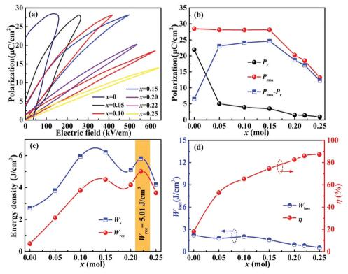
Fig. 6 (a) Unipolar P-E loops for xBMT ceramics at  $E_b$ . (b) Variation of  $P_{max}$  and  $P_r$  as a function of x content. (c)  $W_s$  and  $W_{rec}$ , and (d)  $W_{loss}$  and  $\eta$  versus applied electric field of various xBMT ceramics
