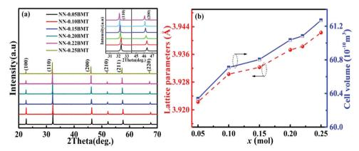
Fig. 1 (a) XRD patterns of BMT-modified NN ceramics. (b) The corresponding Lattice parameters and unit cell volume as a function of x.
