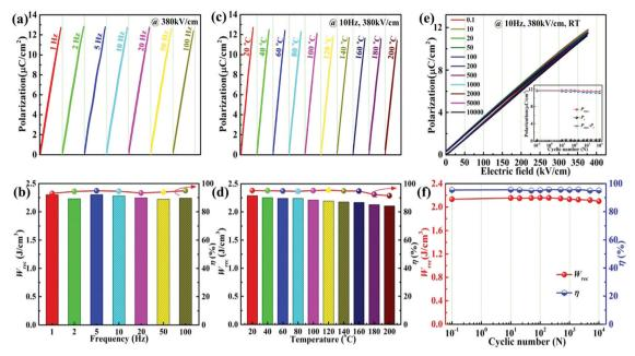
Fig. 8 Unipolar P-E hysteresis loops (a and c) and the corresponding energy storage properties (b and d) for 0.22BMT ceramics at different frequencies and temperatures under different electric fields. The cycle number dependence of (e) unipolar P-E loops and (f) energy storage properties of 0.22BMT ceramics.
