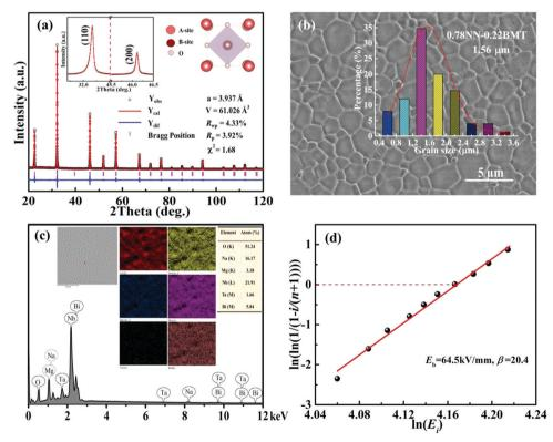
Fig. 2 (a) XRD Rietveld refinement, (b) SEM image, (c) elemental mapping and (d) the Weibull distribution of the  $E_b$  for the 0.22BMT ceramic. The inset of (a) shows enlarged (110) and (200) peaks and XRD Rietveld refinement results of the 0.22BMT ceramic. The inset of (b) is a view of the grain size distribution.
